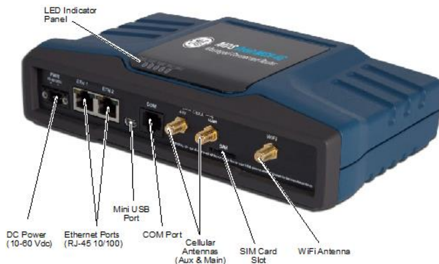
Figure 2-2. MCR Connectors and Indicators (Sample configuration with Cell, WiFi, two Ethernet and one Serial port)
